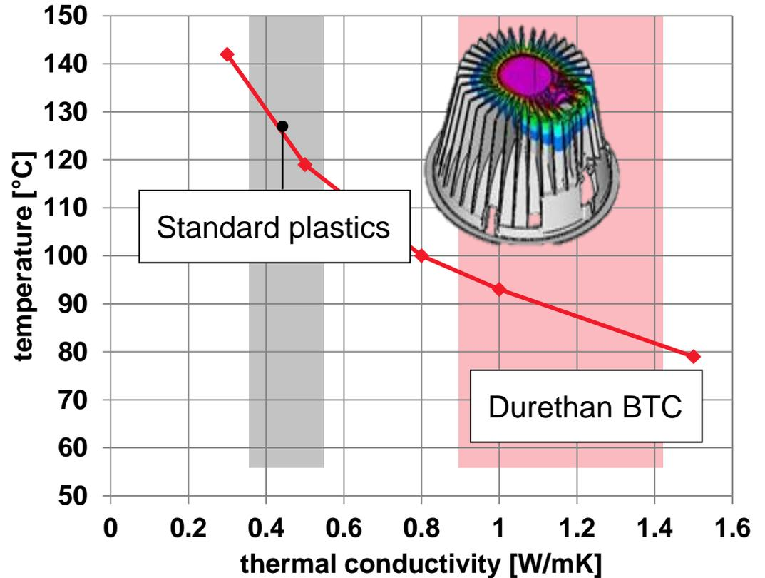
**Exemplary temperature reduction depending on thermal conductivity**
