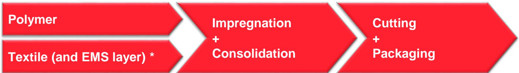
\*EMS layer: Metal mesh (Cu, steel), metal film (Al, Cu, MuMetal), carbon fleece or shielding fleece
