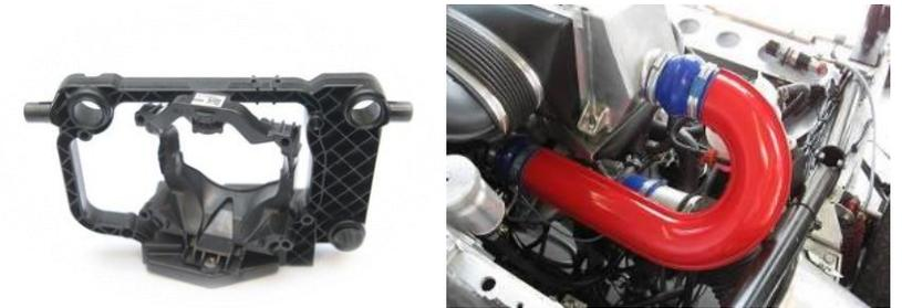
PPA: Curve Light Adjustment, Charge Air Duct
